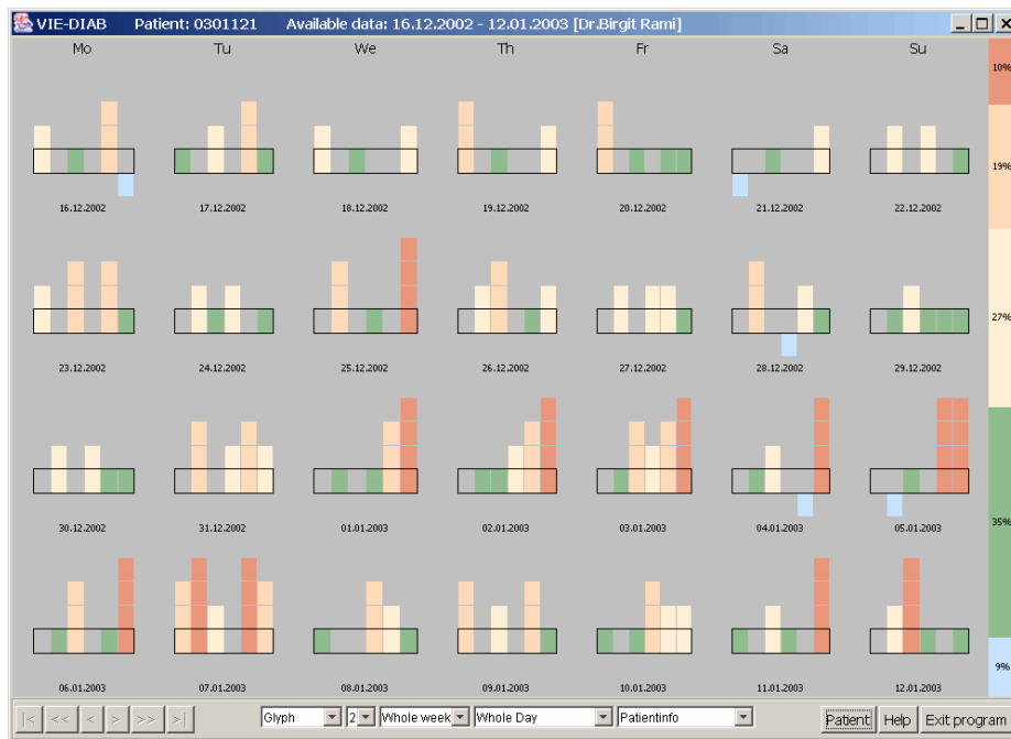
Fig. 1. VIE-DIAB's glyph data display. Serum glucose values are intuitively displayed as glyphs representing one day, 7 multiples in a row, 4 rows per sheet. The relative distribution of the serum glucose categories is displayed in the right margin.
